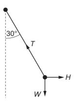
The tension in the string of the pendulum is T. The weight of the pendulum bob is W. The string is held at an angle of  $30^{\circ}$  to the vertical.
