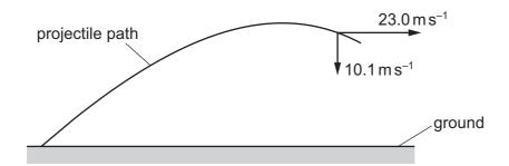
At a certain time, the projectile has a horizontal velocity of  $23.0\,\mathrm{m\,s^{-1}}$  and a vertical velocity of  $-10.1\,\mathrm{m\,s^{-1}}$ .
